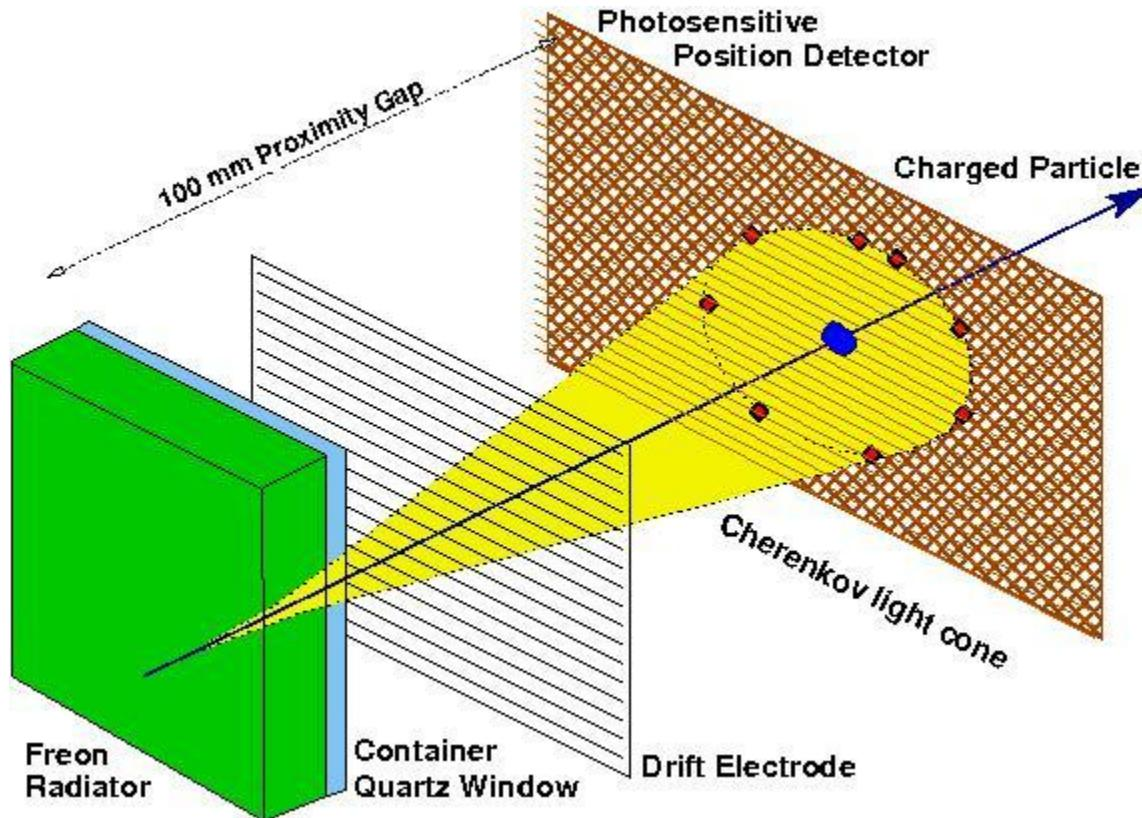
TWO main element: “radiator” and “photon detector”
