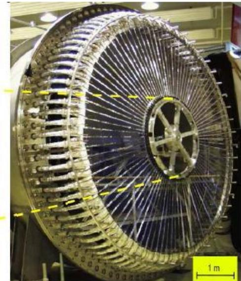
View on the tank of the TOF detector. The ring and central detector, the wedge shaped layer of the ring and the layer with Archimedean spirals of the central detector are shown.
