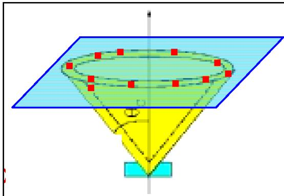
Ring thickness determined by thickness of radiator (gas, liquid)
