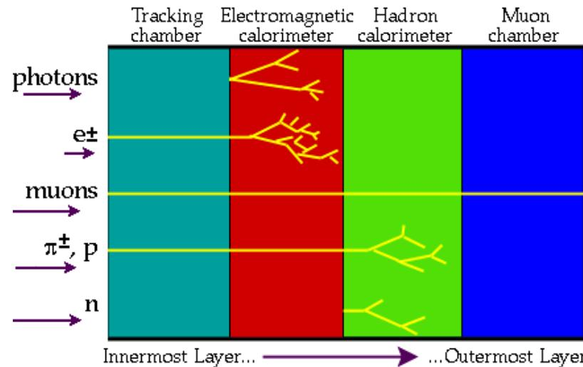
The imprints of different particle types in the different layers of a particle detector
