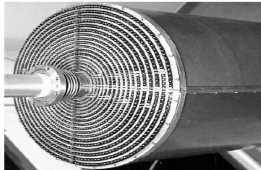
MDC is fitted inside a cylindrical cover made of 1 mm Al-Be and placed inside the solenoid.
