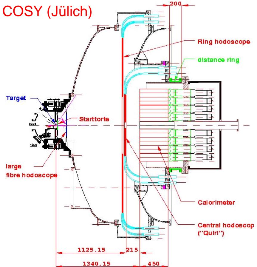
ToF + Tracking information close to interaction point: determination of 4-vectors of produced particles
