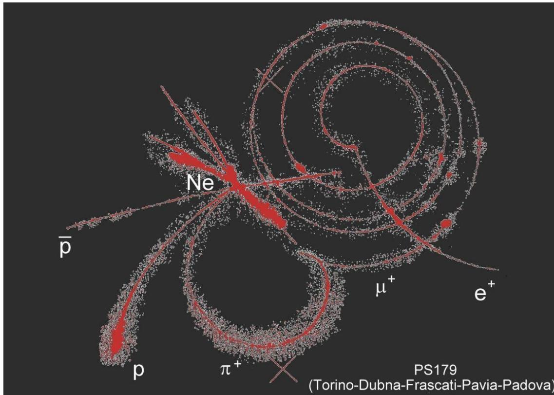
Streamer chamber photo of pion-muon-electron ( $\pi\text{-}\mu\text{-}e$ ) decay chain resulting from antiproton annihilation. The antiproton annihilates with a proton in neon ( $Ne$ ) gas filling the chamber.
