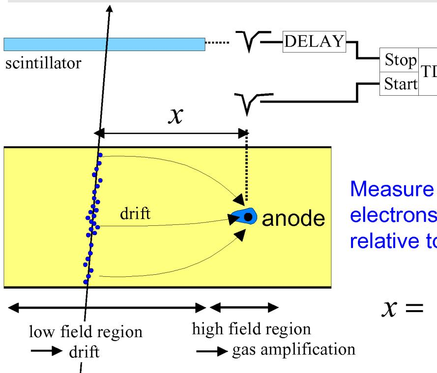
Measure arrival time of electrons at sense wire relative to a time  $t_0$ .
